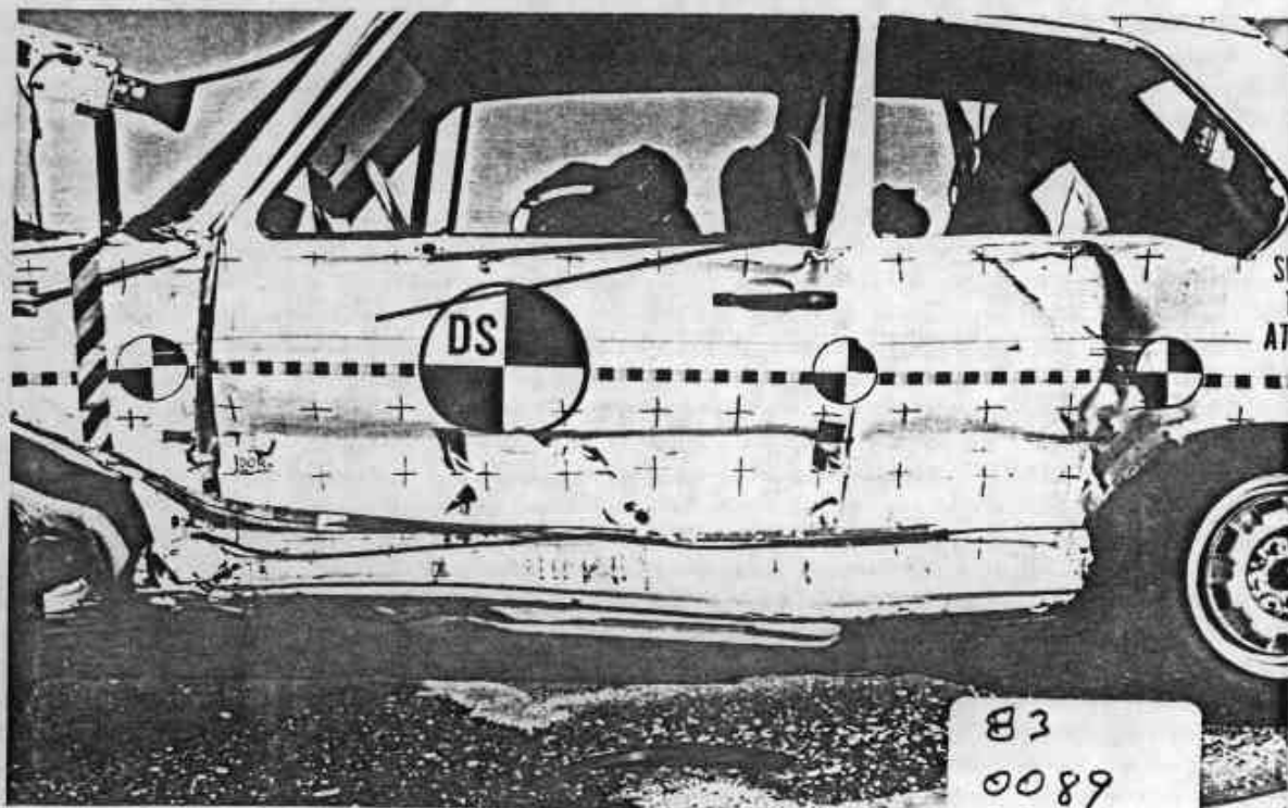
FIGURE A-4. POST-TEST LEFT SIDE VIEW OF VW RABBIT - 26° CRABBED SIDE IMPACTOR TO 1982 VW RABBIT - 28.60 MPH.
