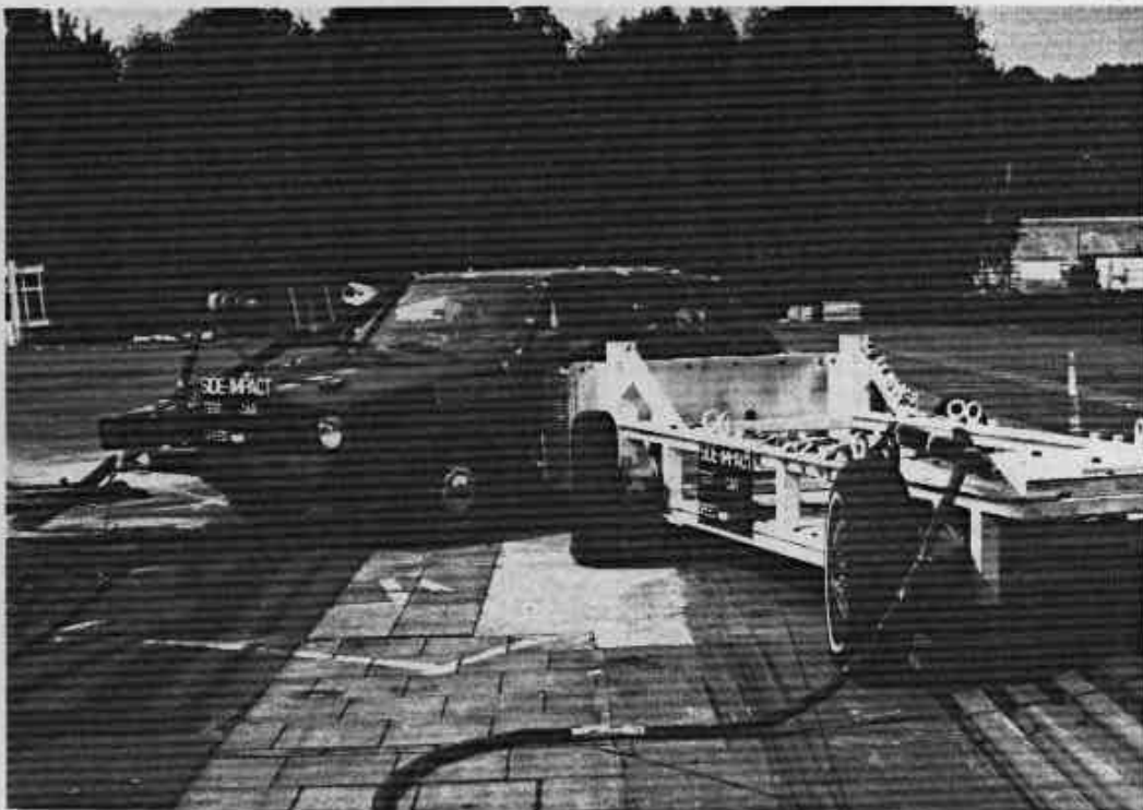
FIGURE 1 : 19° CRABBED BARRIER TEST DEVICE
