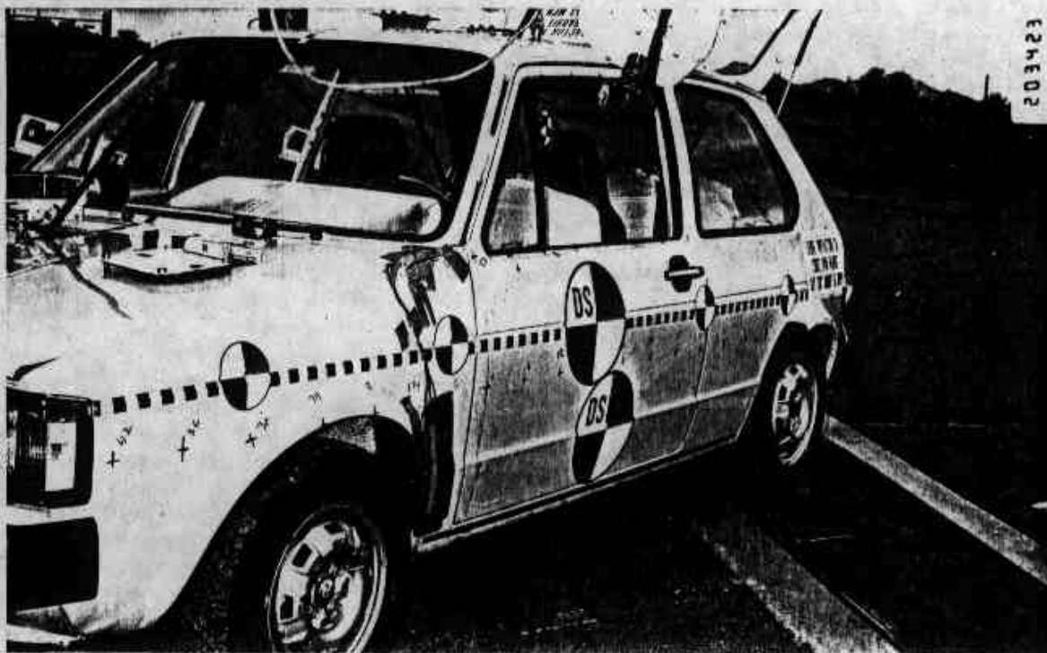
FIGURE A-1. PRE-TEST FRONT VIEW OF VW RABBIT - 19° CRABBED SIDE IMPACTOR TO 1982 VW RABBIT - 53.38 MPH.
