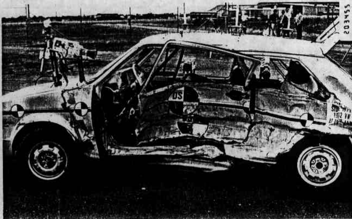
FIGURE A-4. POST-TEST LEFT SIDE VIEW OF VW RABBIT - 19° CRABBED SIDE IMPACTOR TO 1982 VW RABBIT - 53.38 MPH.
