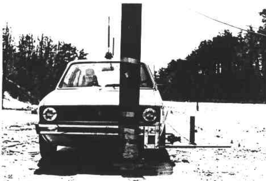
Figure 5. Pretest Photograph of Test Vehicle Shown in Contact with Surrogate Luminaire Support, Front View
