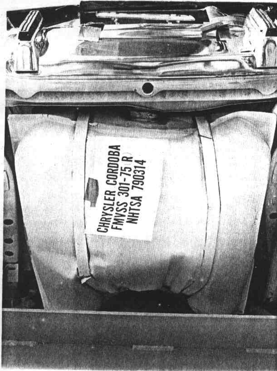
Figure 3-2. Post-test Fuel Tank.
