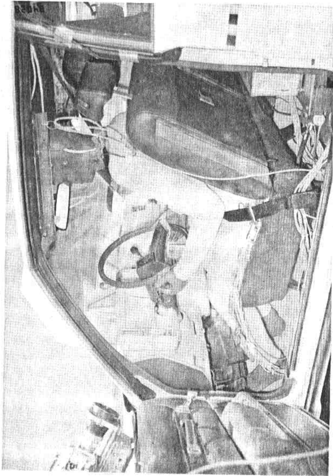
Figure 3-1. Pre-test View of Driver Dummy - 1978 Chevrolet Monte Carlo Two-Door Sedan - NHTSA 780113.
