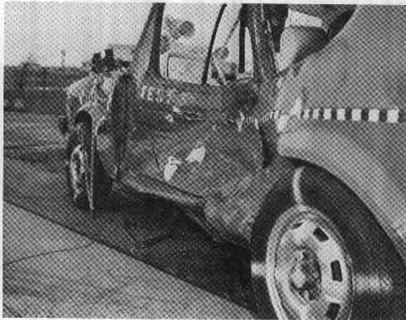
SIDE DAMAGE ON V.W. RABBIT
