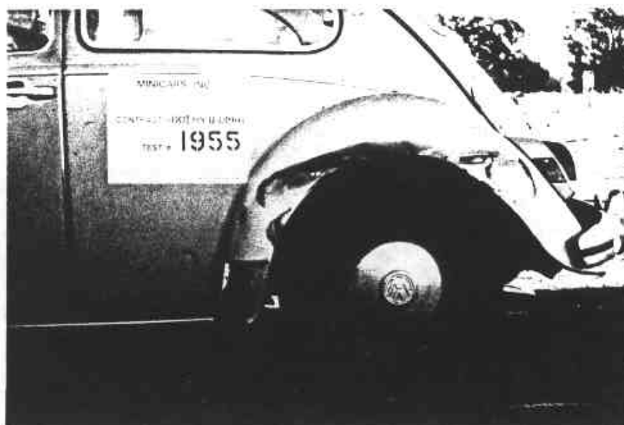
FIGURE 4. PRE-TEST LEFT HAND SIDE FENDER DAMAGE
