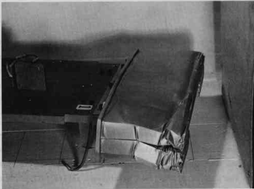
(b) AFTER 34-mph BARRIER IMPACT
