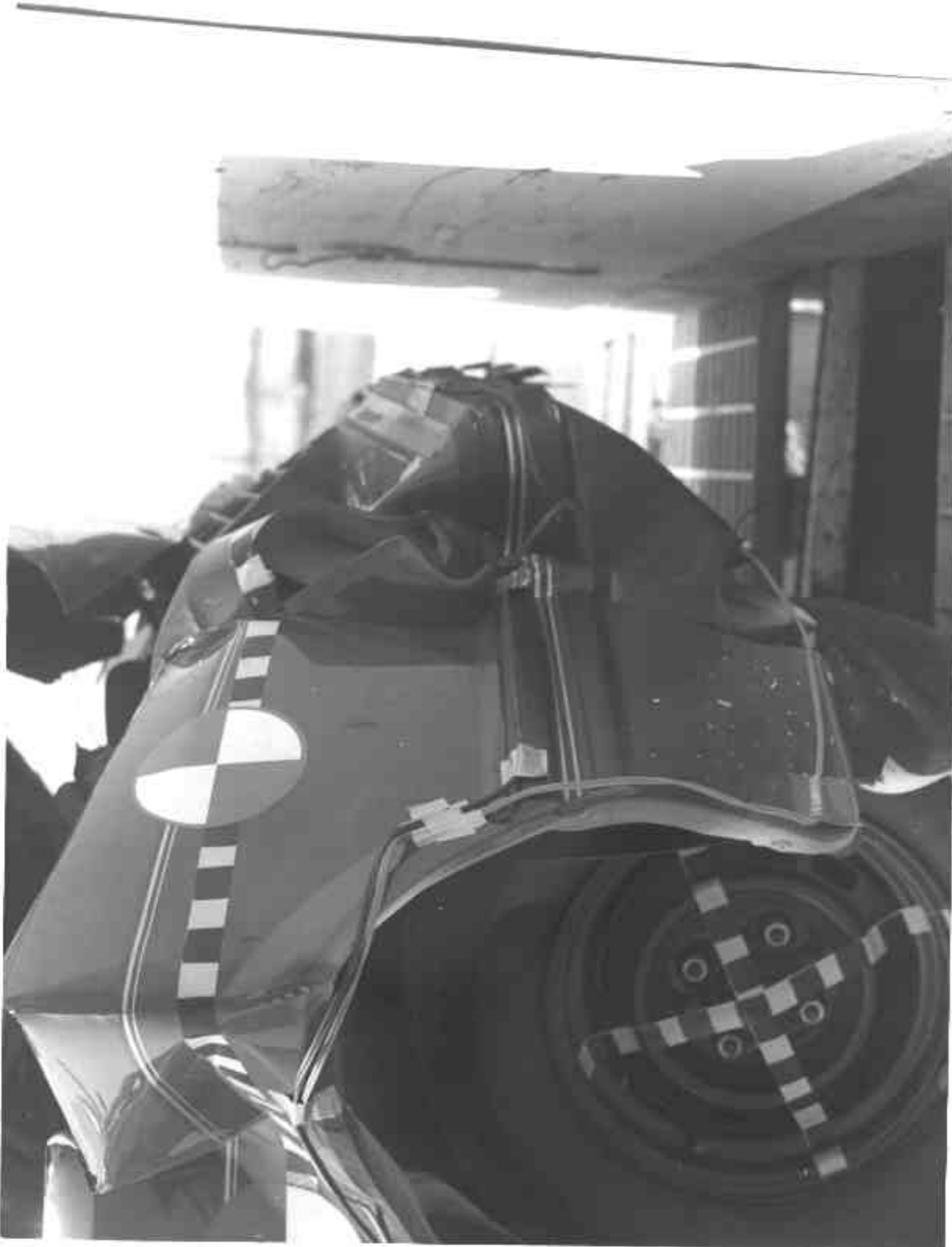
Figure 2-5. Post-test Right Side View of Impact Area.
