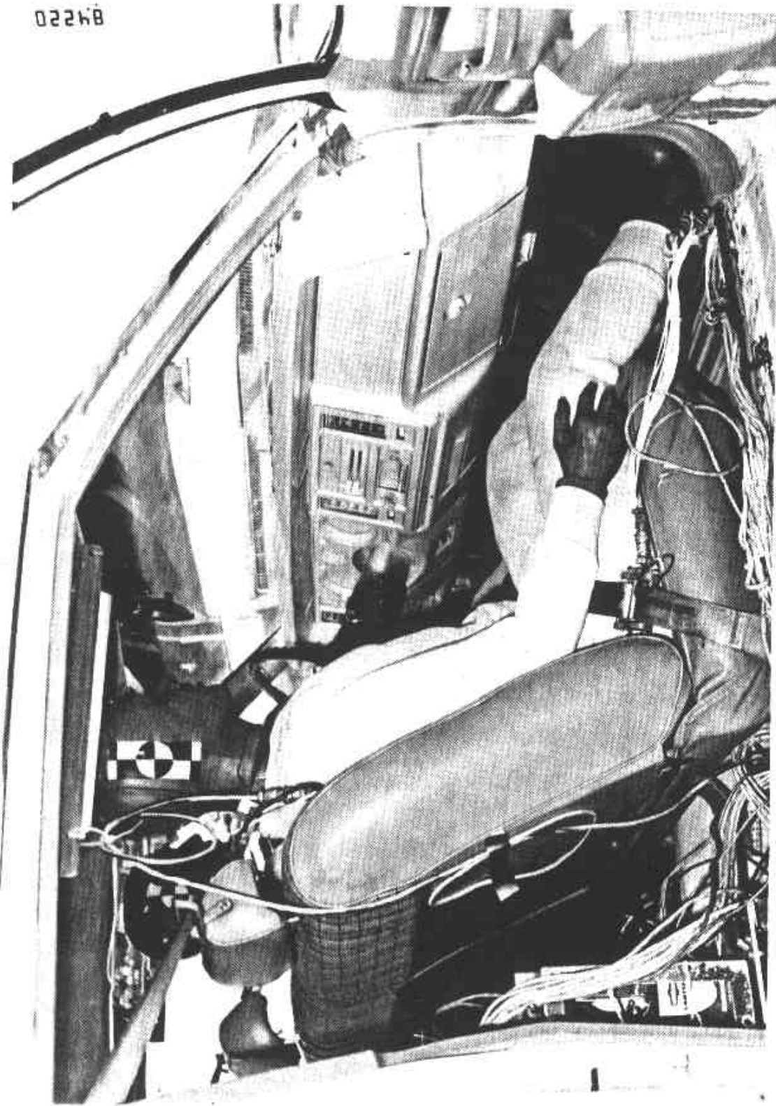
Figure 3-2. Pre-test View of Passenger Dummy - 1978 Buick LeSabre Two-Door Sedan - NHTSA 780109.
