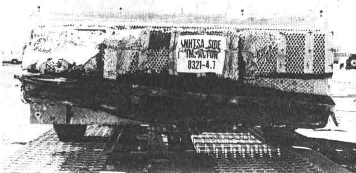
b) Post-test Side Impactor
