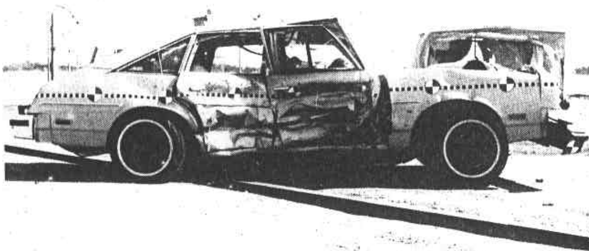
a) Post-test Oldsmobile Cutlass
