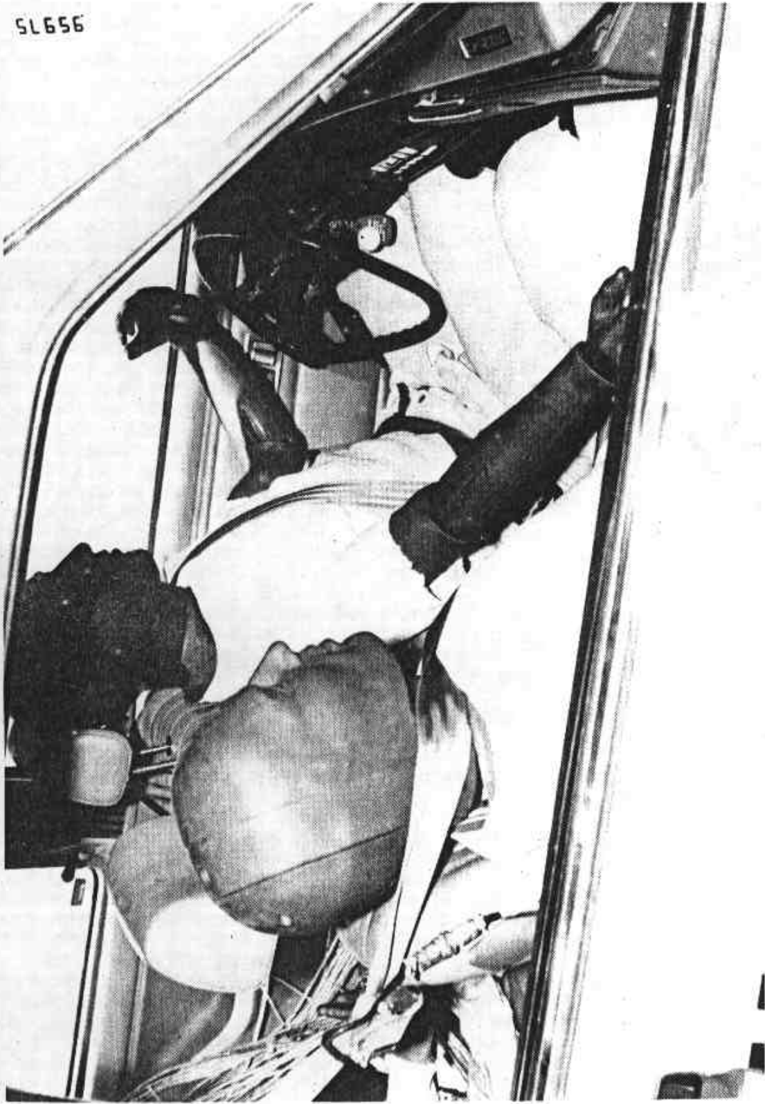
Figure 4-3. Post-test Driver Dummy Position - 1979 Plymouth Champ 2-door Hatchback - NHTSA No. 790522.
