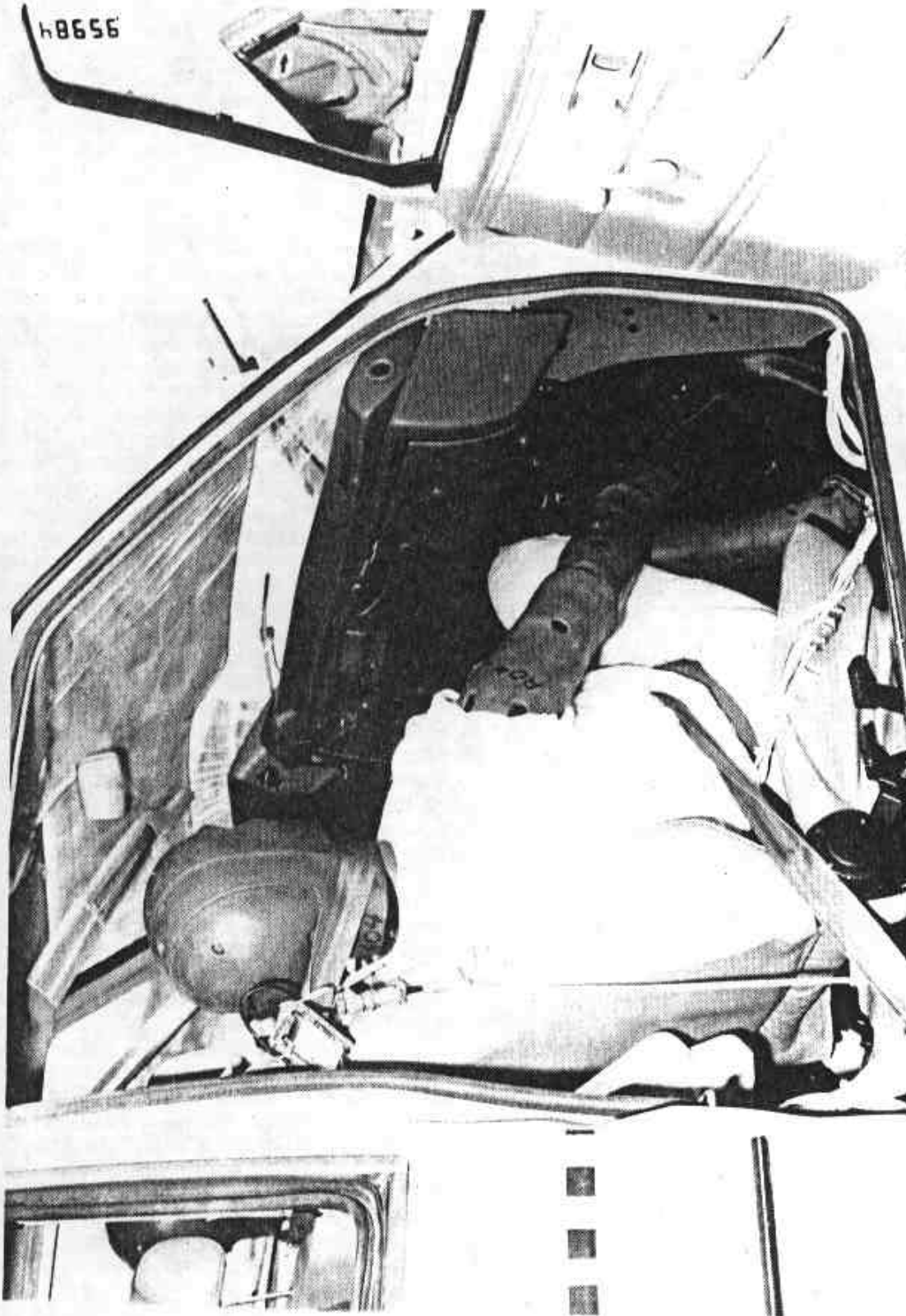
Figure 4-6. Post-test Passenger Position - 1979 Plymouth Champ 2-door Hatchback - NHTSA No. 790522.
